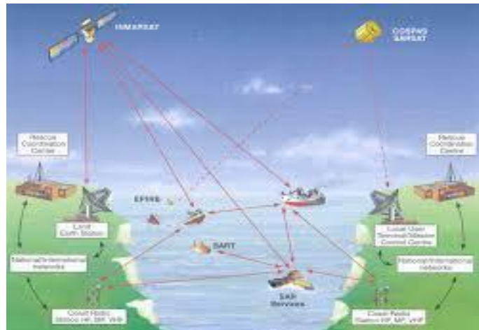
Fig. 2 Architectural image of GMDSS
